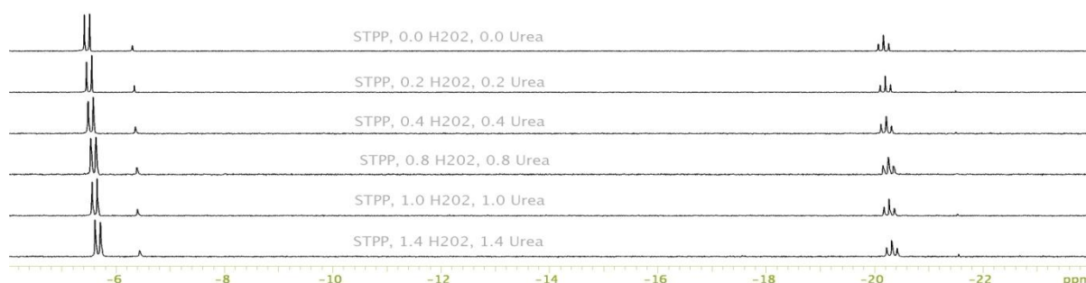
Figure 5a. ^{31}\text{P} nmr spectra showing the simultaneous addition of both \text{H}_2\text{O}_2 and Urea to a fixed STPP concentration.
